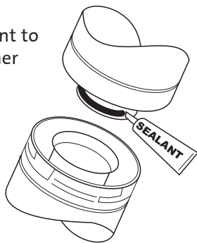
Figure 5. Exhaust Restrictor Plate installation.
